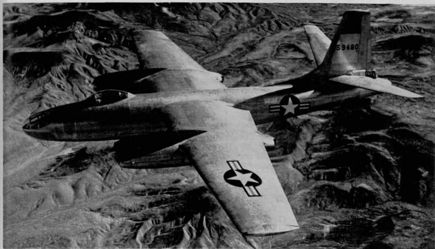
North American's B-45 "Tornado" is a light bomber in the 550 miles per hour class. With a ceiling of over 40,000 feet, it carries a bomb load of 20,000 pounds over a combat radius of 800 miles.
